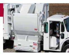
The SB8200 Split-Body Side Loader was specifically designed to address customer needs for a single collection vehicle that can haul multiple commodities and eliminate the need for a second truck.
